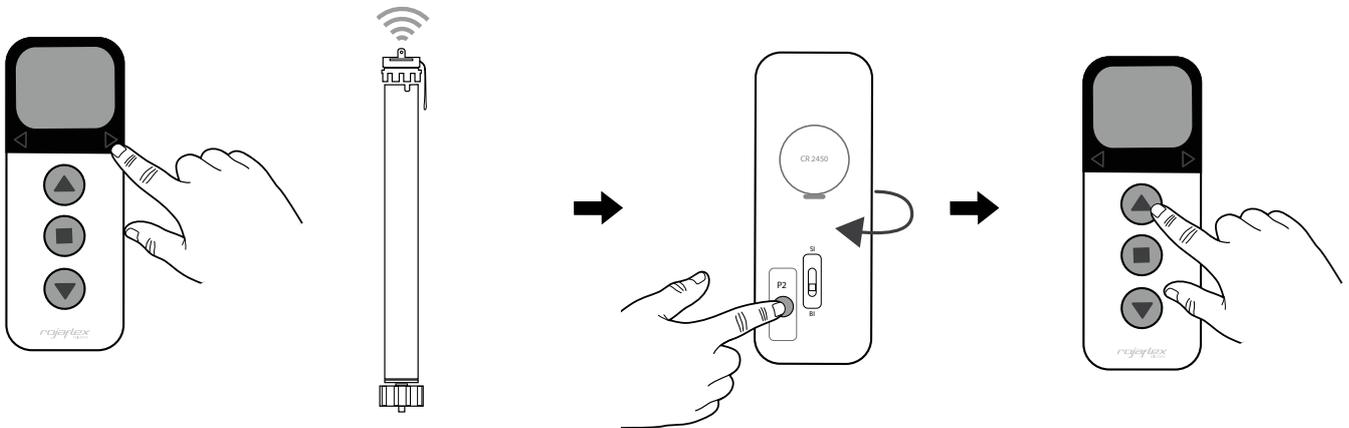
First select the desired channel by pressing the K1 (or K2) key (the channel highlighted in black is selected).
