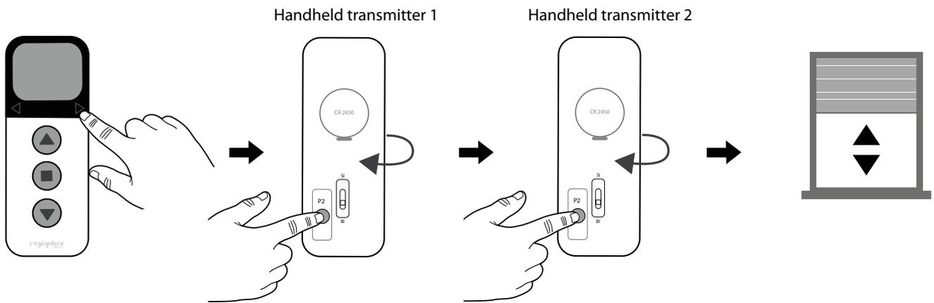
At an ALREADY programmed station, select an already programmed channel by pressing the K1 (or K2) key.
