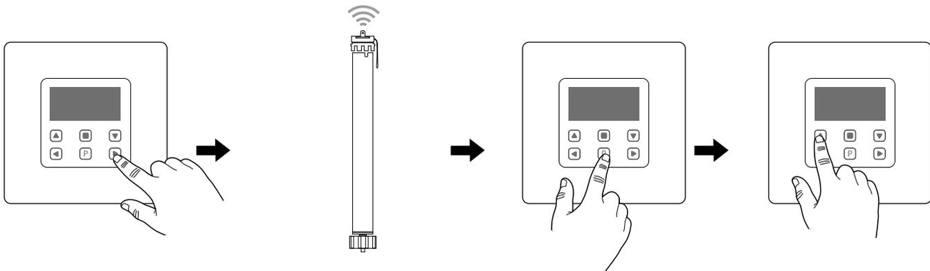
Select the desired channel by pressing the K1 (or K2) key (the channel highlighted in black is selected).
