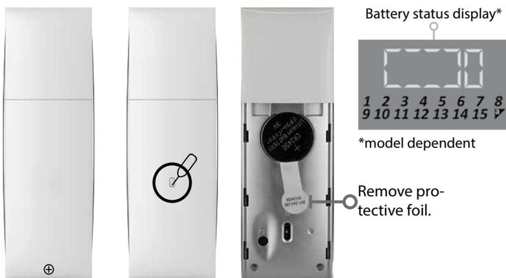
The battery is (depending on the transmitter model) supplied loose or already installed and secured against discharge with a protective film. To replace/insert the battery, open the rear cover by pressing lightly downwards\*, remove the protective film and insert the battery into the battery compartment with the + (plus) side facing upwards as shown. Then close the rear cover again.
