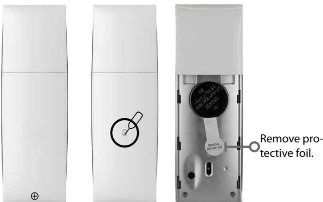
The battery is (depending on the transmitter model) supplied loose or already installed and secured against discharge with a protective film. To replace/insert the battery, open the rear cover by pressing lightly downwards\*, remove the protective film and insert the battery into the battery compartment with the + (plus) side facing upwards as shown. Then close the rear cover again.
