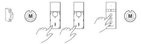
1.7 \*Conditionally check the direction of rotation of the motor! When pressing the OPEN button, the awning must CLOSE!
