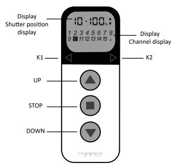
15-channel handheld transmitter RHS15-W
