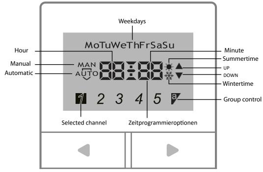
The changeover from summer to winter time takes place automatically according to fixed days. The current date must be set correctly during initial programming!
