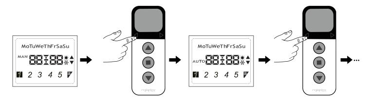
MAN Manual mode Press and hold the K1 key. After approx. 5 seconds, the display changes from "MAN" to "AUTO".
