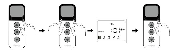
Select the desired channel by pressing the K2 (or K1) key (the channel highlighted in black is selected).
