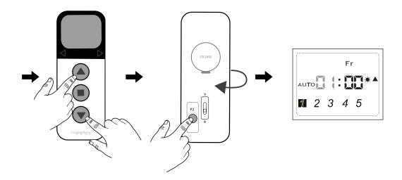
Proceed as for programming the automatic OPEN time. As soon as the hour and the minute for the DOWN time have been set, press the P2 key again.
