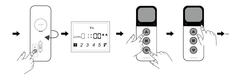
After the desired time programming option has been selected, press the P2 programming key once.
