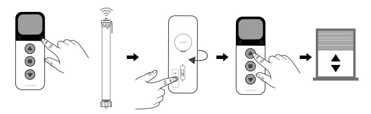
Press the K1 (or K2) key and select the desired channel (the channel highlighted in black is selected).
