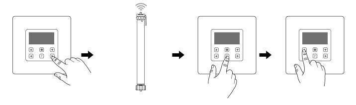
Select the desired channel by pressing the K1 (or K2) key (the channel highlighted in black is selected).
