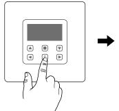
Press the P2 programming button 3 times on the wall transmitter that has already been programmed.
