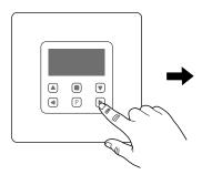
At an ALREADY programmed station, select an already programmed channel by pressing the K1 (or K2) key.
