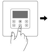
Then press the P2 programming button once on the wall transmitter to be reprogrammed.
