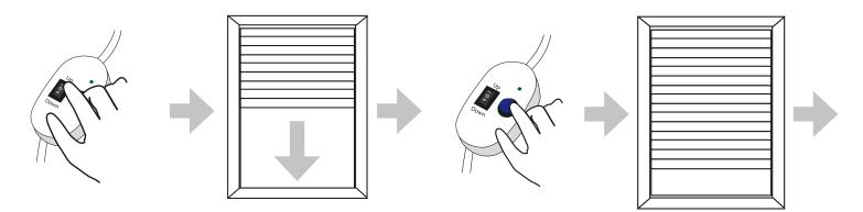
As soon as the roller shutter has reached the desired upper end position, release the programming button and set the UP/DOWN switch to the DOWN position.
