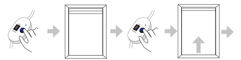
Shortly before the shutter has reached the desired upper end position, press the programming button on the ESK-01 or on the motor head.
