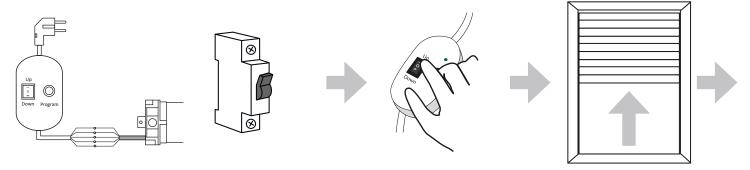
Connect the motor according to the connection diagram (page 10-11) to the ESK-01 or a suitable pushbutton and switch on the power supply.
