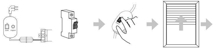
Connect the motor to the ESK-01 or a suitable pushbutton according to the connection diagram (pages 11-12) and switch on the power supply. Press the UP/DOWN switch to the UP position.
