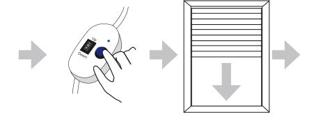
Then press the UP/ DOWN switch to DOWN position within 0.5 sec.
