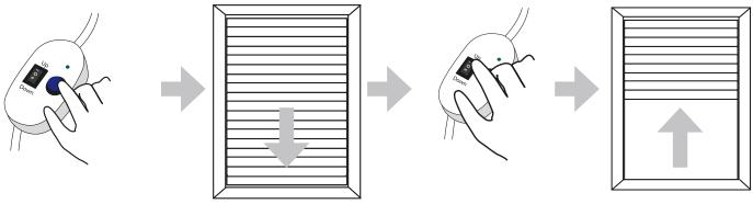
Programming key press = Roller shutter moves down.
