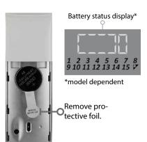
The battery is (depending on the transmitter model) supplied loose or already installed and secured against discharge with a protective film. To replace/insert the battery, open the rear cover by pressing lightly downwards\*, remove the protective film and insert the battery into the battery compartment with the + (plus) side facing upwards as shown. Then close the rear cover again.
