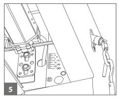
For manual operation of the motor in case of power failure a crank handle (Crank not included) into the crank eyelet and open or close the roller shutter with the crank.
