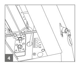
Fix the mounting plate of the crank joint to the masonry (the box).
