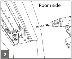
Drill passage for the crank rod through the masonry (the box).
