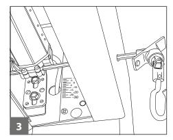
Insert the crank rod through the wall into the emergency manual gearbox of the motor.
